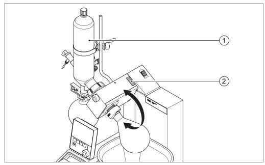
Fig. 32: Adjusting the immersion angle
