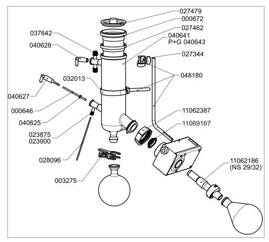
Fig. 53: Glass assembly C
