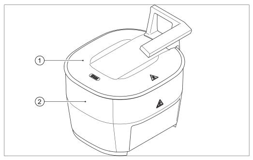
Fig. 5: Heating Bath B-305 with cover
