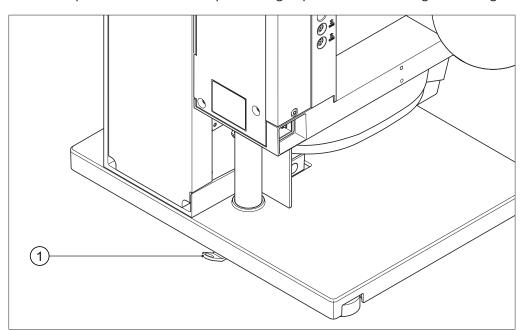
Fig. 6: Earthquake fixing
