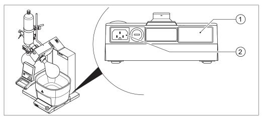
Fig. 23: Power supply connection on heating bath base
