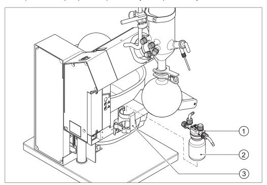
Fig. 12: Mounting the Woulff bottle on the Rotavapor
