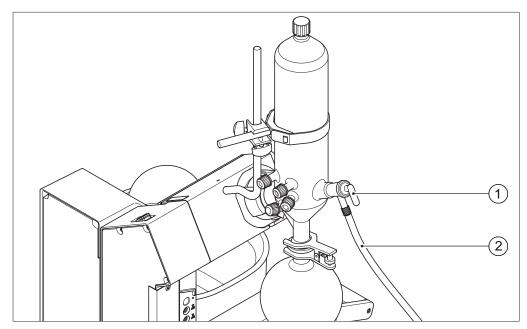
Fig. 42: Cooling condenser with glass stopcock and backfeed tube
