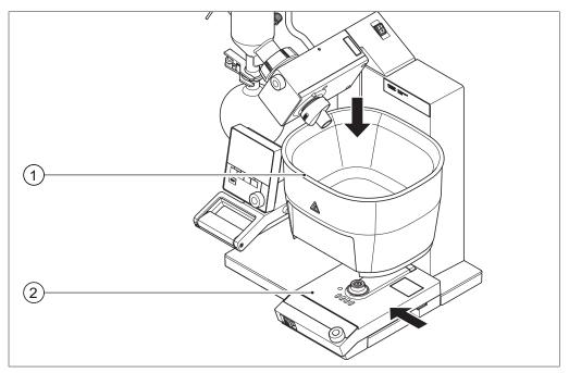
Fig. 17: Heating Bath B-305 and Heating Bath B-300 Base
