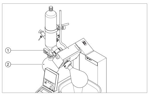
Fig. 33: Fitting the receiving flask
