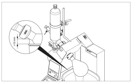
Fig. 34: Clearance between evaporating flask and edge of heating bath
