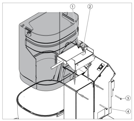
Fig. 20: Fitting the splash guard on the Rotavapor
