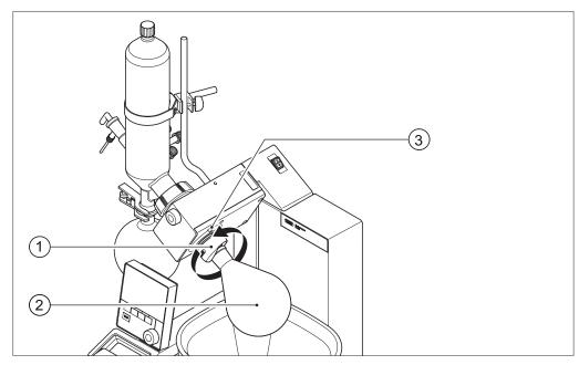
Fig. 43: Evaporating flask on Rotavapor R-300
