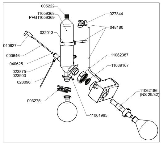
Fig. 51: Glass assembly V
