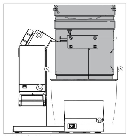
Fig. 21: Aligning the splash guard
