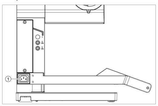
Fig. 22: Power supply connection on Rotavapor R-300
