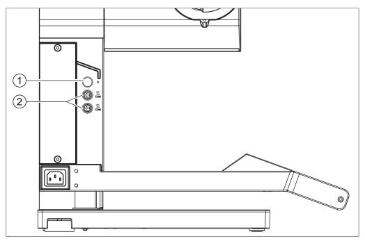
Fig. 26: Communication cable connections on Rotavapor
