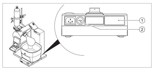
Fig. 49: Fuse in heating bath base
