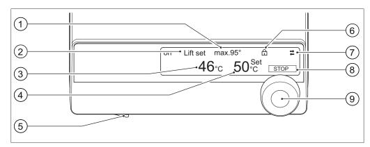
Fig. 3: User interface of Heating Bath B-300 Base
